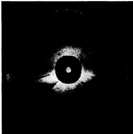
FIG. 6-2.—A shadow on the PPI caused by a large airplane that blocks the radar beam. This airplane is flying just below and slightly behind the one in which the photograph was taken. The radar signal from the airplane is lost in the bright spot at the center of this picture.
