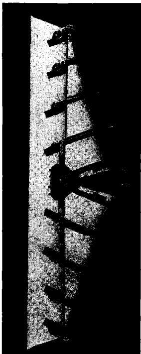
FIG. 7-21.—Robinson scanner. This is a view of the specially shaped throat of the Robinson scanner, which is used to illuminate the reflector of a height finder. It can be seen mounted in front of the reflector at the right in Fig. 7-20. A rotating waveguide feed is attached to the coupling shown in the center. (Courtesy of American Machine and Foundry Company.)
