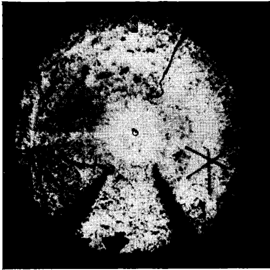
FIG. 6-1.—The aircraft wheels block the radar beam and produce two wedge-shaped shadows on the PPI.
