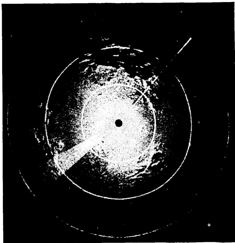
FIG. 3-13.—Southern California mountains from 13,000 ft with a 3-cm production radar. The range circles indicate 5-mile intervals.
