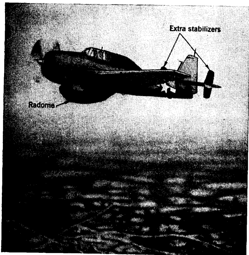
FIG. 6-5.—The design of a radome to house an 8- by 3-ft parabolic reflector underneath the airplane presented a difficult problem in streamlining. Two additional vertical stabilizers were required.
