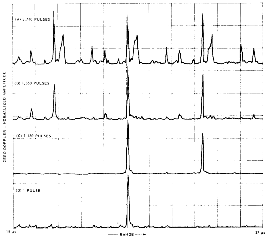
Figure 11.24 Effect of geometric programming on land clutter echoes. (A) 3740 pulses, 150 kHz—no programming; (B) 1550 pulses, geometric programming—no clutter decay; (C) 1130 pulses, geometric programming—12.8 \mu s clutter decay; (D) single 0.15 \mu s pulse. (Courtesy of A. Chwastyk)
